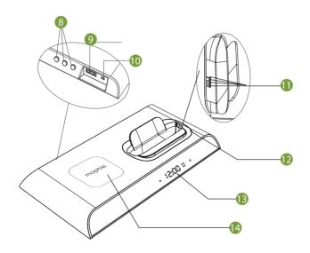
The mophie powerstation wireless dock can be powered using the supplied wall plug. The wireless charging power bank can be charged by placing it upright on the charging dock. The charge time is 3-4 hours.
