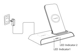
When the smartphone is on the dock, LED Indicator 1 will be white. When the Power Bank is on the dock, LED Indicator 2 will be white.
